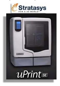
The uPrint has a 8 x 6 x 6 build envelope, a .010" print resolution and uses ABS material.
